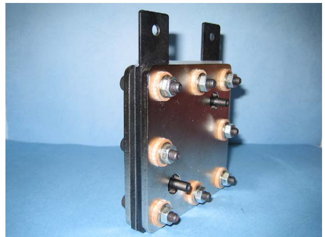
Fig. 7. Prototype one-cell PEM fuel cell stacks with titanium bipolar plates.
