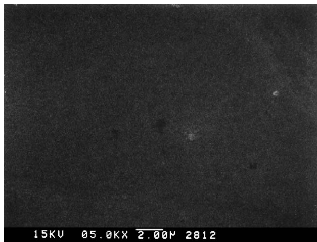
Fig. 1. SEM image of pure titanium bipolar plates without surface modification.
